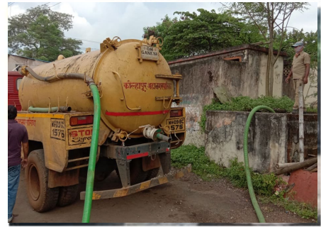
Tanker Decanting Septage
