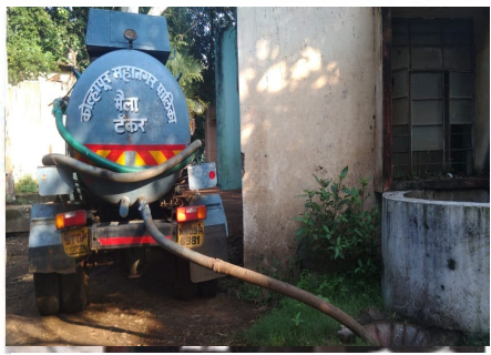
Decanting of Septage in Progress at Jayanti Nallah pumping station, Kolhapur, Maharashtra, India
